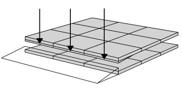
When you connect a **platform** and a **ramp**, remove the **Ramp Adjuster** from the ramp, and use it to adjust the platform as shown here:
