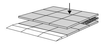
Locks in platform: S-Lock is mounted on the top layer.
