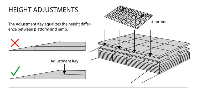
When you connect a platform and a ramp, remove the Ramp Adjuster from the ramp, and use it to adjust the platform as shown here:
