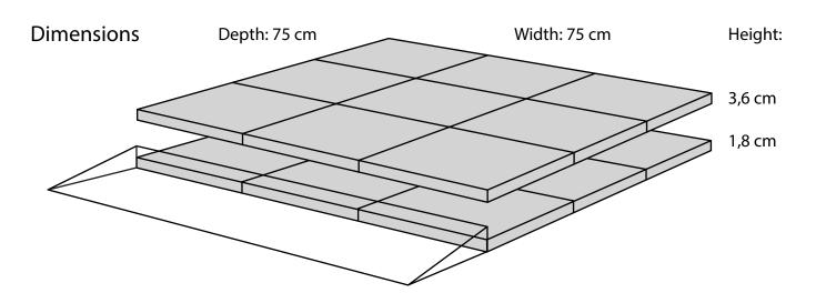
Build together with the Ramp Kit 1, the height can be adjusted up to 5,2 cm
