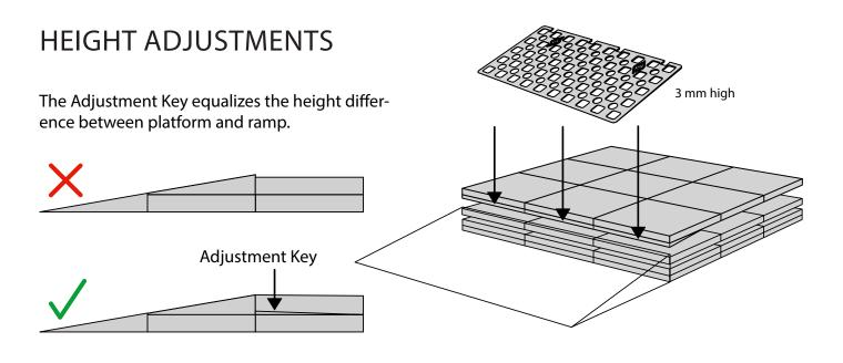
When you connect a platform and a ramp, remove the Ramp Adjuster from the ramp, and use it to adjust the platform as shown here:
